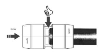
After mounting pull the pipe forcibly by hand to ensure correct installation.
