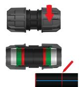
.2 Push the PE pipe into the fitting, until it meets the internal stopper.
